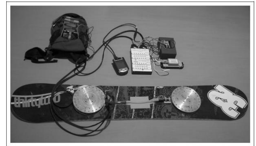
Figure 2. Entire force measurement system mounted on the test snowboard including two force plates, data logger, bridge amplifier unit, connector box, battery pack and backpack.
